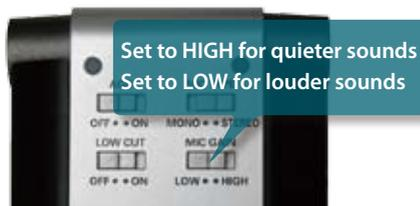
The R-09 allows you to set the basic mic gain in order to utilize its microphone's features to their fullest. By setting this first, the gain is optimized, the recording level is easier to adjust, and, of course, the result is a better recording.
